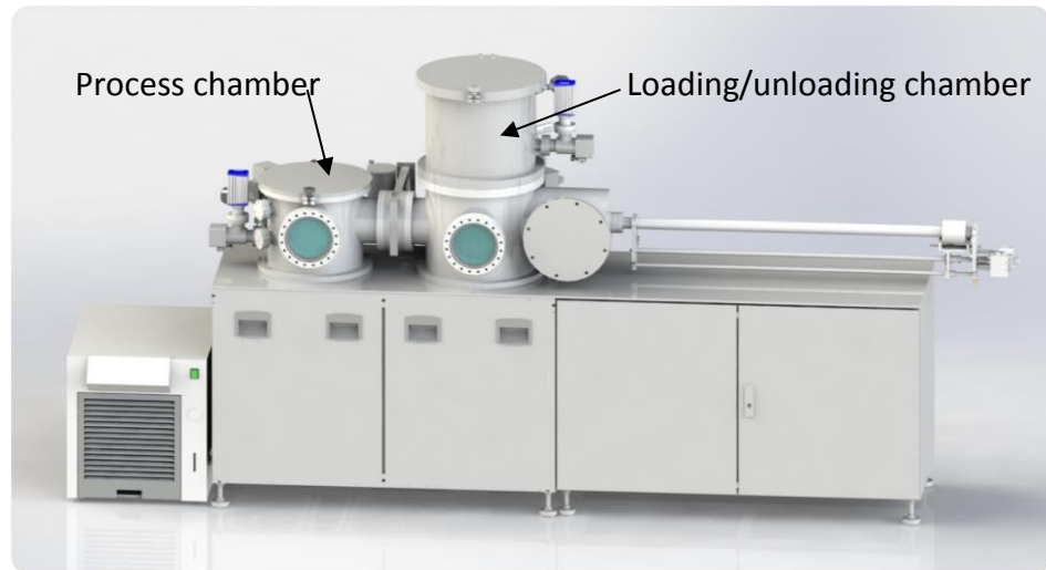
Fig. 1 Conceptual image of Pilot vacuum deposition tool SAF L-EM
